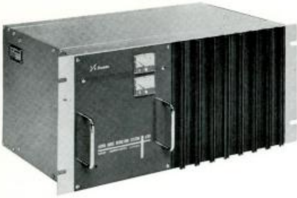
Figure 3. The standard Dolby A301 unit. It contains two processors, each suitable for record or replay.
